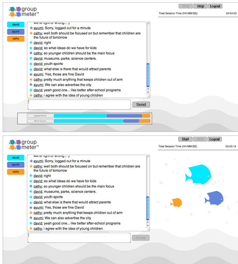
Figure 1. The GroupMeter chatroom with two feedback designs: (a - top) bar graphs, (b - bottom) school of fish. Length of bars and fish size and position represent team members' word count and proportions of agreement word use.
